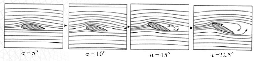
Flow separation takes place from <u>the trailing edge</u> at thicker airfoils than leading-edge stall
