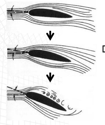
Flow separation takes place over the entire top surface of the airfoil after <u>occurring</u> <u>at the leading edge</u>
